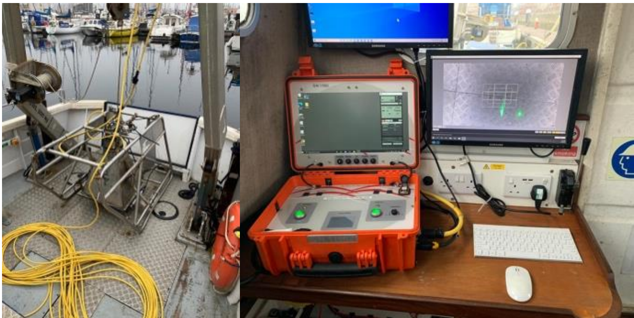
Plate 2 Left: OEL's ROVTech camera system equipped with CLOC. Right: OEL's ROVTech camera system topside computer control station.
